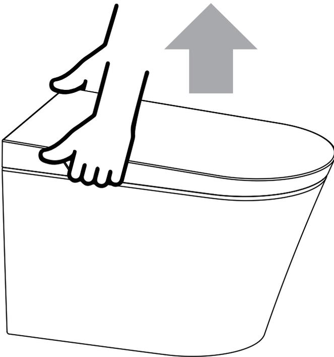
5. Remove the power cord from the back inside and set to the outside of the toilet for easy access after bolting down the toilet.
