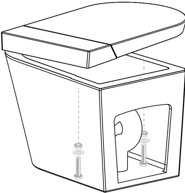
Note: Do not over tighten as you may crack the porcelain/base. If there is still movement once tightening is done, shims may need to be used to account for an unlevelled floor.
