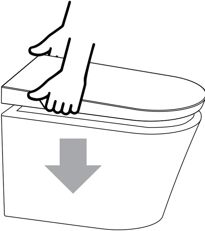
11. Replace the bidet seat by lining it up and pushing down gently on the top part of the seat.
